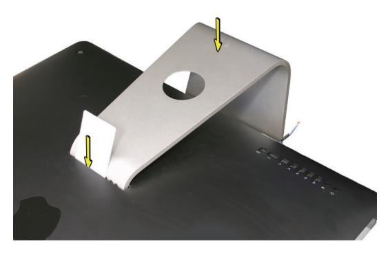
Insert the card as far as it will go, and press the stand down until you hear a click—the audible cue that tells you that the stand is locked into place.
